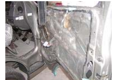
Anti-rust coating for inside door
