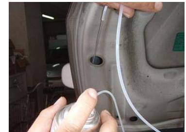
Anti-rust coating under hood
